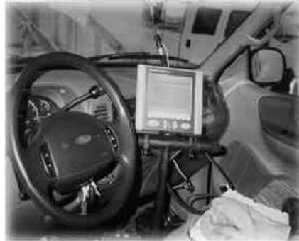
Figure 2: The ice thickness monitor mounted in the cab of the pick-up truck gives the operator a real time read-out of ice thickness.
