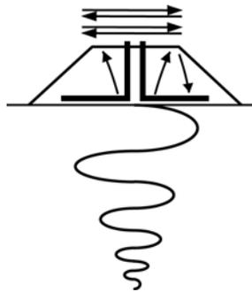
(b) Currents generated on antenna shield bounce back and forth emitting signal.
