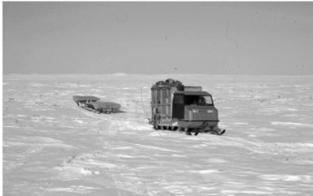
*Figure: 1-5 GPR system being used to survey potential pipeline routes in the Canadian Arctic (1975).*
