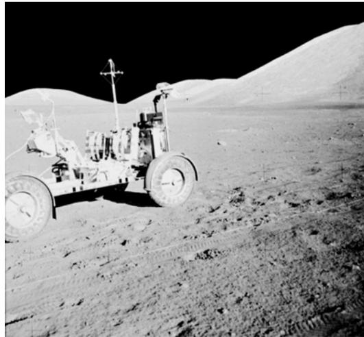
*Figure: 1-4 The surface electrical properties experiment carried out on Apollo 17 used a 3 component vector receiver mounted on the lunar rover and a dual axis multi-frequency dipolar antenna laid out on the surface to sound the subsurface.*
