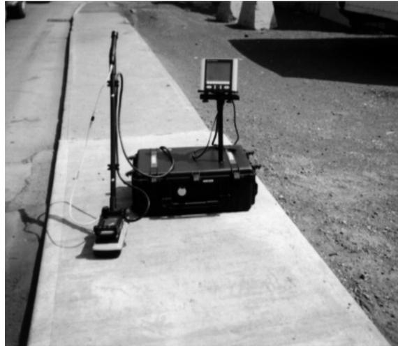
*Figure 1: Conquest on the test sidewalk*
