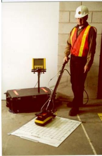
*Photo of Conquest GPR system designed specifically for imaging concrete. Data are acquired on a predefined survey grid.*
