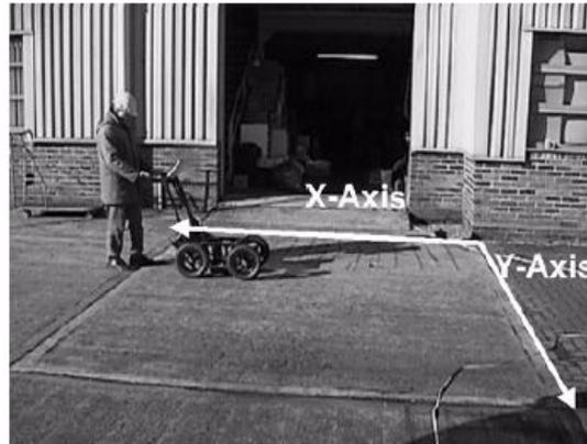
Figure 1: Photo of the test slab with axes indicated. A Noggin 1000 SmartCart maps the area.
