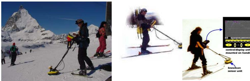
*Photos of a compact, lightweight SnowScan GPR designed specifically to measure snow depth and combine with GPS positioning.*
